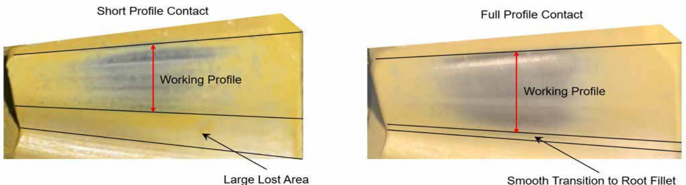
Figure 16: Roll test results V0 profile shift (left) and positive pinion and gear profile shift (right).
