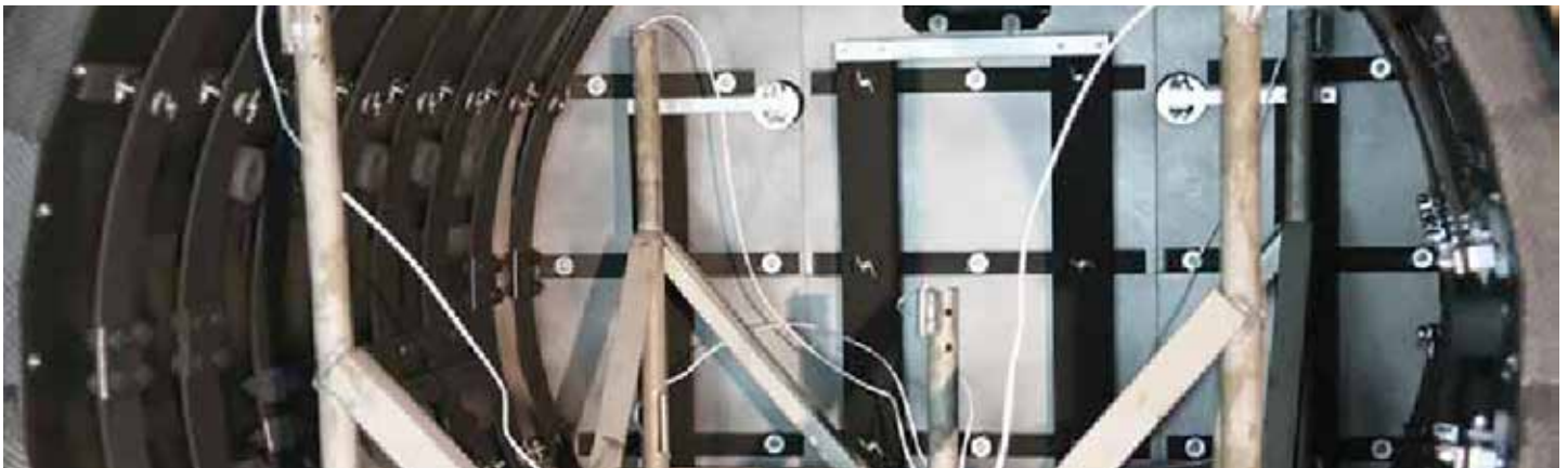
Figure 2: Typical rack used for industrial furnaces, showing the location of thermocouples at each corner of the work zone, and at the geometrical center [7].
