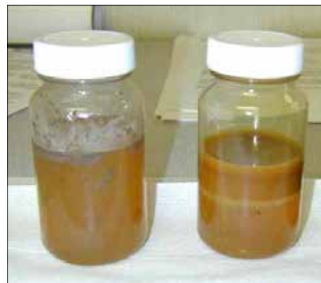
Figure 3: In use samples of polymer quenchant badly contaminated with coolant from the prior machining operation. A new solution would be a clear, slight amber color.
