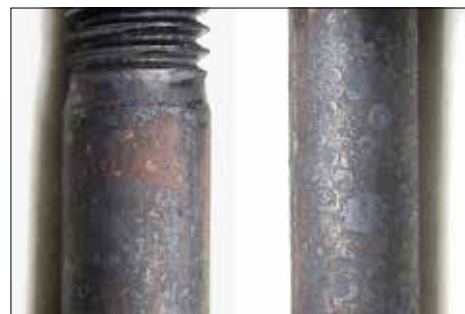
Figure 4: Rusting and caustic burn resulting from improper cleaning and rinsing of parts prior to heat treatment.
