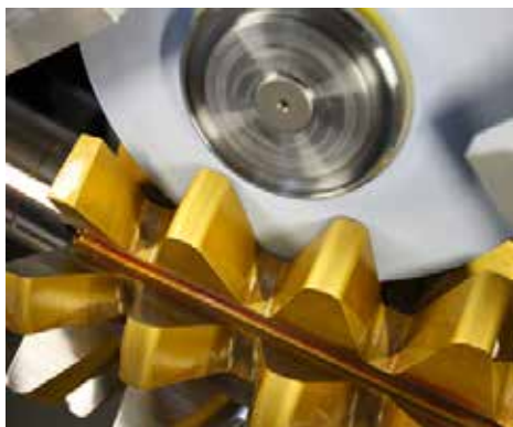
The dimensional accuracy and surface quality of a gear component are key to an efficient transmission of power and smooth operation. (Courtesy: Haas Multigrind)
