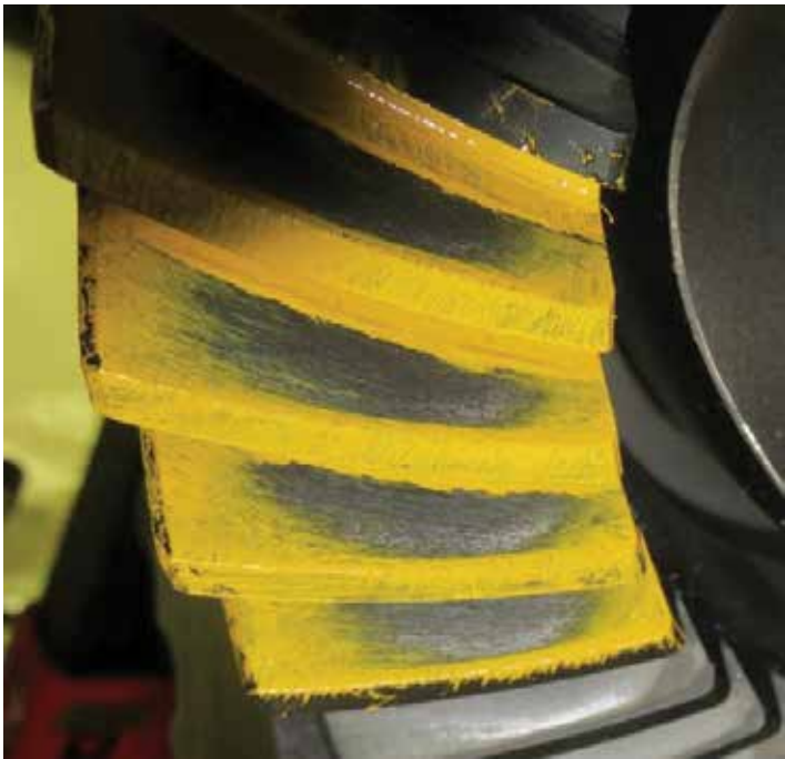
Figure 5: An example of acceptable shape and configuration of contact pattern under a low load.
