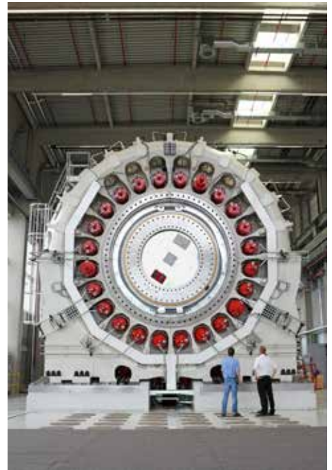
Assembly of the MSTR load unit. (Courtesy: Renk)
