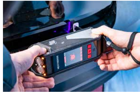
The new wireless, blue light, non-contact Calipri C15 tool gives manufacturers greater flexibility when inspecting fit and finish in production and assembly lines. (Courtesy: Hexagon MI)
