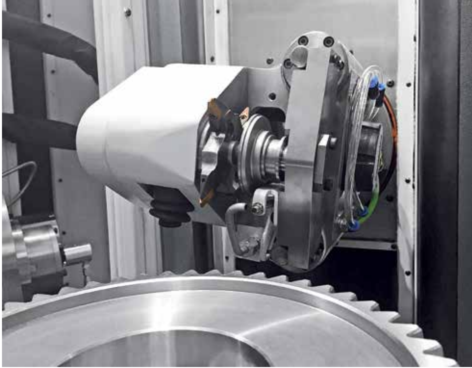
Chamfer Contour Milling in parallel to gear hobbing on the Gleason 400HCD does not add cycle time and is ideal for trucksize gears.
