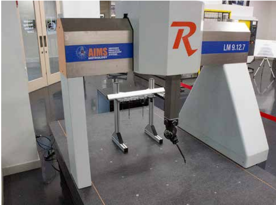
AIMS Metrology has equipped its Revolution Series LM coordinate measuring machine (CMM) with a Renishaw 5-axis REVO 2 head and the new SFP2 probe. (Courtesy: AIMS)
