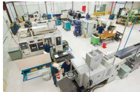
Forest City Gear's new facility is now dedicated almost solely to the precision turning and milling operations needed to produce precision gear blanks. (Courtesy: Forest City Gear)
