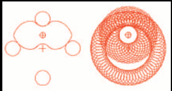
Figure 1 — Two-tooth partially conjugate prolate epitrochoid spur gear reducer of parallel input/output shafts for ratio R=2:1 .
