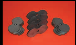
Figure 1 — Two-tooth partially conjugate prolate epitrochoid spur gear reducer of parallel input/output shafts for ratio R=2:1 .
